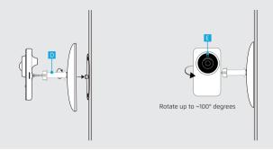
Press the foot of the camera on the white plastic mounting plate (The metal ring does not have to be placed back). Screw the stand of the camera back on the foot and tighten it. It is possible to rotate the camera up to ~100° degrees.
